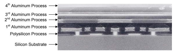
Photomicrograph of the SXRD panel silicon backplane in cross section.
